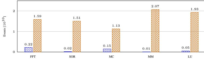
Figure 6: Empty FPU cycles (■) and CPU cycles (■) count for each test of the SciMark2.0 benchmark.
