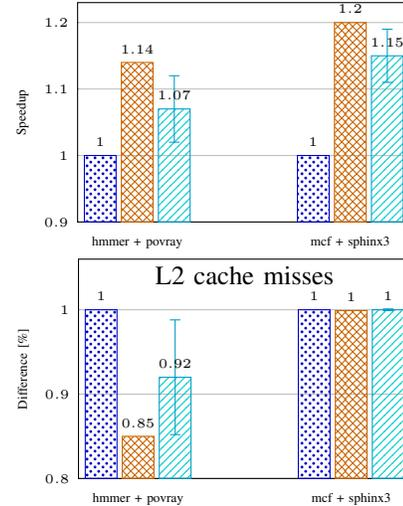
Figure 7: Spec.CPU speedups (top) and cache miss differences (bottom) using an intentionally inefficient baseline (1) versus using BulldOver to improve performance (2) or letting the default OS scheduler do the job (3).
