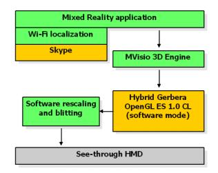
Figure 4: Architecture overview: improved framework with software rendering. Dark boxes are third-part products.
